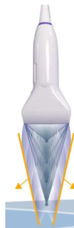
*Radiation force created by SonicTouch™. The shear wave is amplified along a Mach cone (yellow). The distance traveled is increased, thus minimizing acoustic energy used.*
