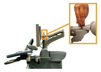
For transportation, put the monitor in its lower position and rotate the screw clockwise in order to lock the monitor in this position.
