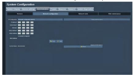
The system can be configured with a specific IP address and network setting, with a cable connected or can be automatically configured in DHCP mode.
