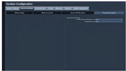
In this section, you can configure the limit duration of the prospective clip capture, for contrast mode and for the other modes.
