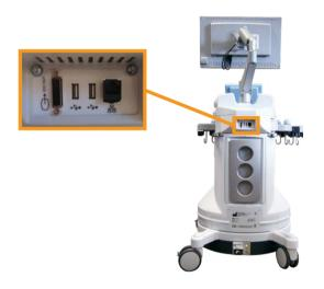
An external monitor which supports DVI capability may be connected to this port.
