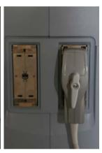
When disconnecting the transducer, turn the lock handle counterclockwise to unlock the connector and then hold the connector and pull it straight out.
