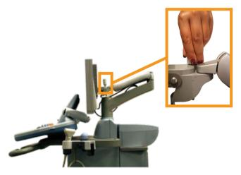
For transportation, put the monitor in its lower position and rotate the screw clockwise in order to lock the monitor in this position.
