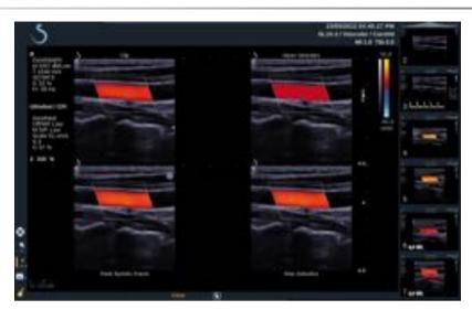
• **Spectrogram** displays the image on the top and the spectrograms underneath.
